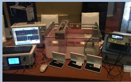
HFO-690 whole setup , including a fiber optic controller, an oscilloscope, an amplifier, a transducer, a fiber hydrophone.
